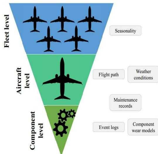
Fig. 1. Inputs to the predictive MRO planning system, shown at approximate level of relationship to the aircraft systems.
