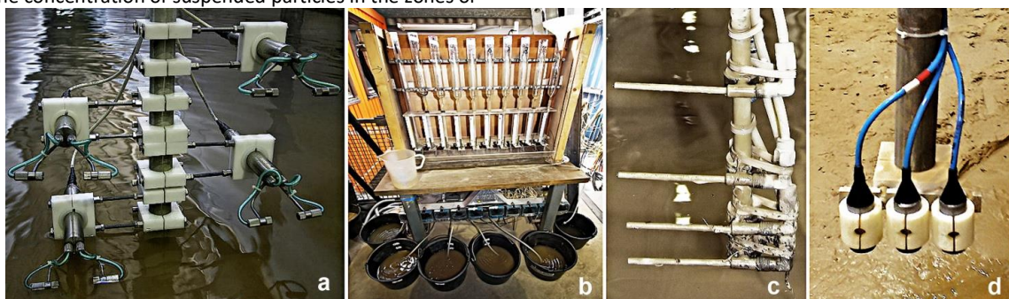
Fig. 3. Suspended sediment concentration meters: a - turbidimeters; b – multi-channel pump TSS; c – water intake gateways of the pump; d – sensors of the ABS profiler
